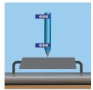
The Remotely Operated Vehicle (ROV) runs above the subsea pipeline. By the two-electrode probe assembled on ROV, the potential between the probe and a remote electrode, and the potential gradient in close proximity of the pipeline, are measured. Every time an exposed anode is met along the pipeline, a direct contact measurement is taken. The two recorded profiles allow to calculate the potential profile of the pipeline and to localize the coating defects.
