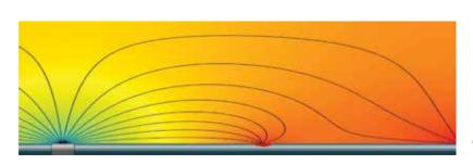
Finite Element Methods (FEM) are used to model the electrical field around the pipeline and close to coating defects. Modelling allows to correctly interpret the inspection results. In case of buried pipelines, the electrical field is modelled considering the burial depth and the sea mud resistivity.
