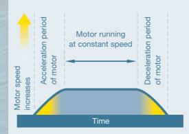
The 520Di can be set to "ramp" up to full speed at the start of a dose and ramp down to zero speed at the end. The slope of each ramp can be independently adjusted. Ramping aids accuracy and allows filling to start and stop at speeds which avoid splashing or foaming, but still allows the highest speed to be used for the main part of the dose: filling is faster. End-of-dose drips are easily avoided using the pump's anti-drip feature: a momentary direction reverse at the end of each dose.
