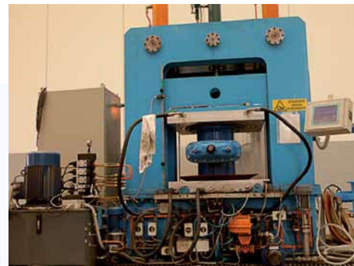
collaudo saracinesche | gate valve testing
