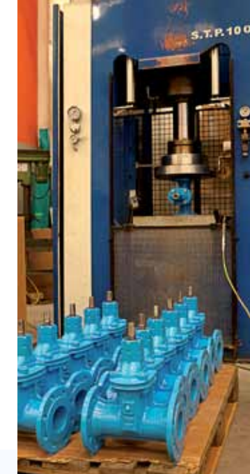
collaudo saracinesche | gate valve testing
